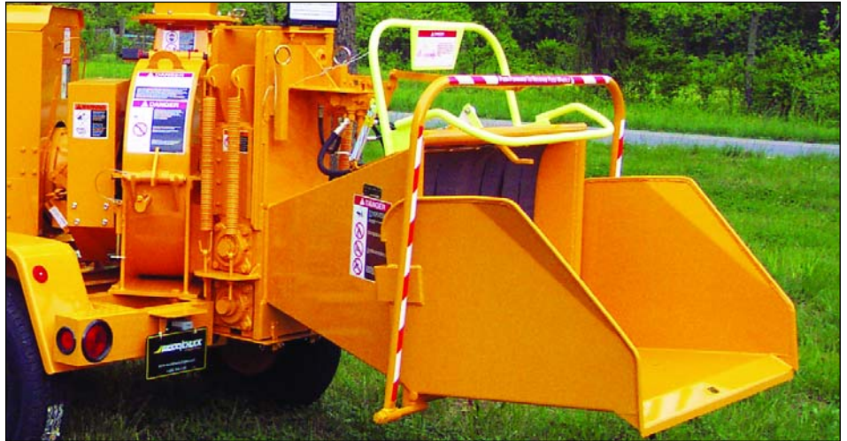
Wood/Chuck developed the patent pending "Panic Bar," painted yellow above, to provide a dedicated, durable mechanism to stop the controlled feed system, and to lock the system out, in an emergency situation.
