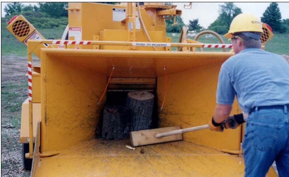
Bandit's wooden push paddle is a simple, expendable tool to help the operator resist the temptation of reaching into the infeed chute to push small pieces.
