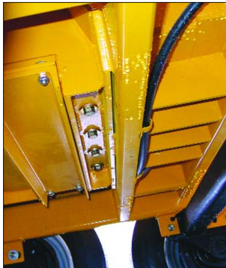
Woodsman chippers are equipped with a removable access panel in the chipper housing that allows access for changing, turning and adjusting the four-sided anvil.
