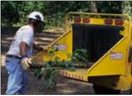
Vermeer's upper feed control bar, combined with the bottom feed stop bar, provides a means for the operator to stop the feed rollers.
