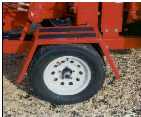
Morbark's chippers have non-slick pads on all fenders to prevent the operator from slipping when climbing onto the chipper during maintenance.
