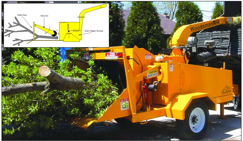
The hydraulic feed wheel on Woodsman chippers can be raised from either side of the machine.
