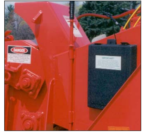
Morbark lock pins lock the chipper drum or disc when changing knives, and when raising the top feed wheel for maintenance.
